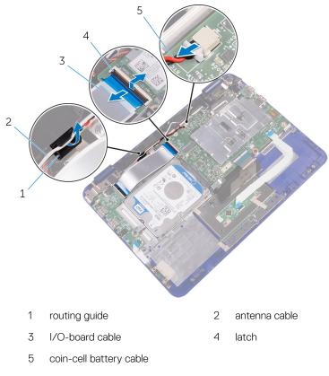
4 Turn the I/O-board cable over to expose the coin-cell battery.
