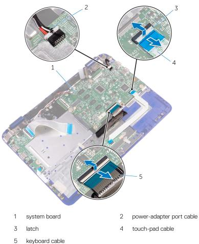
8 Remove the screw that secures the system board to the palmrest and keyboard assembly.
