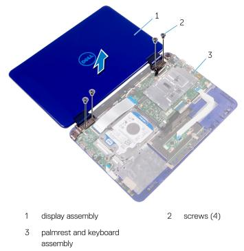
12 Lift the display assembly off the palmrest and keyboard assembly.
