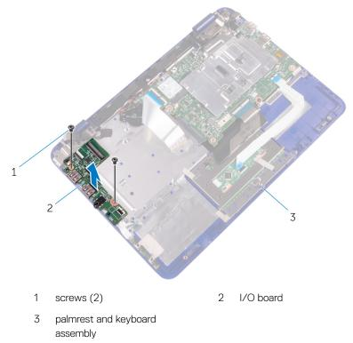
**3** Lift the I/O board off the palmrest and keyboard assembly.
