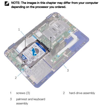
**5** Remove the screws that secure the hard-drive bracket to the hard drive.
