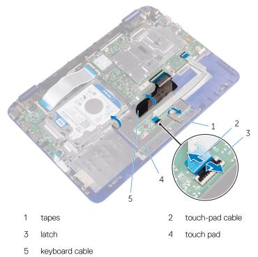
**4** Remove the screws that secure the touch pad to the palmrest and keyboard assembly.
