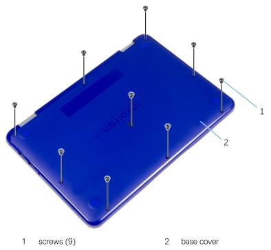
**4** Using a plastic scribe, pry the base cover from the palmrest and keyboard assembly.
